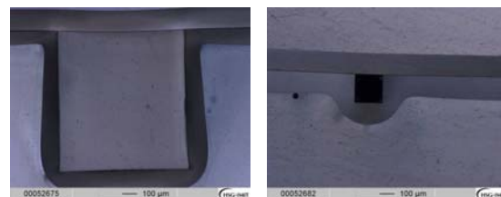
Fig 5. Sealed 1 mm cavity (left) and 200 \mu\text{m} channel (right). Both samples are bonded to the edge of the channel and show none to negligible deformation.
