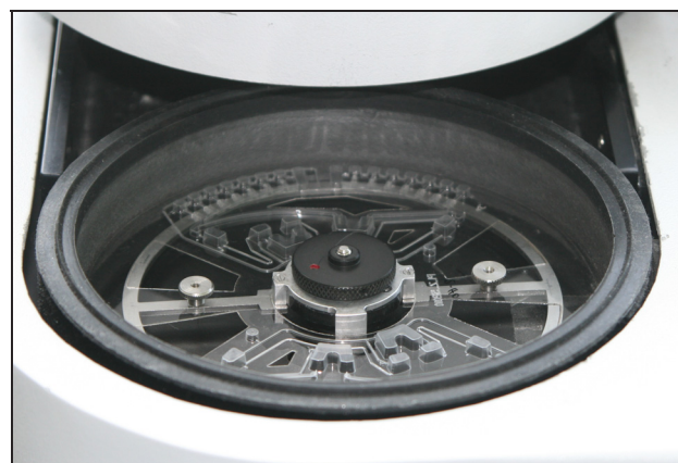
Fig 2: Microfluidic foil disk for food pathogen detection placed in the real-time PCR thermocycler (Rotorgene 2000, formerly Corbett Research; now Qiagen).
