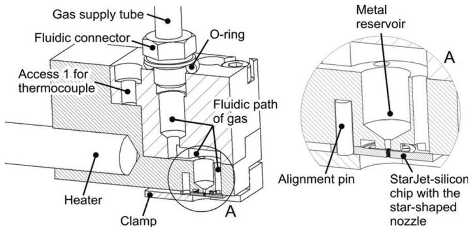
pneumatic and thermal control elements. These are described in detail in the experimental section at the end of this article. Before presenting the results in detail, the working principle of the StarJet dispenser is described, which is based firstly on the centering of liquids inside a star-shaped nozzle, and secondly, on the propagation, elongation, and the break-off of the liquid column within the nozzle.
