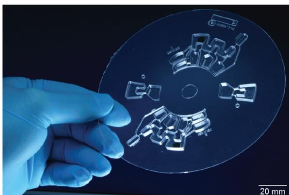
**Fig. 3** LabDisk, replicated by the µTSL process featuring two independent *GTM* structures, each with three buffer chambers designed for a bind-wash-elute protocol used in magnetic bead based DNA purification.
