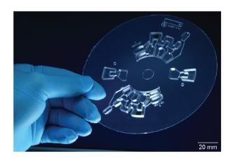
Fig. 3 LabDisk, replicated by the  $\mu$ TSL process featuring two independent *GTM* structures, each with three buffer chambers designed for a bind-wash-elute protocol used in magnetic bead based DNA purification.
