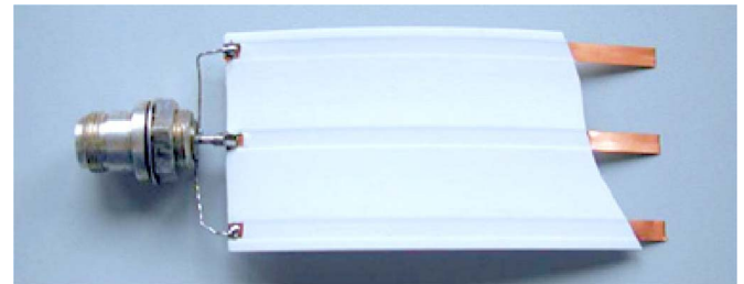
Fig. 1. Flat ribbon cable with a characteristic impedance of approximately 200 \Omega in air. The cable is buried, e.g., in soil, and the dielectric properties of the surrounding soil influence the characteristic impedance along the cable, which affects wave propagation and causes partial reflections.
