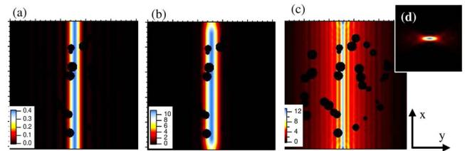
Fig. 2. (Color online) Cross sections of unstained spheres and of ideal light-sheets in the center of the sphere cluster. (a) Gaussian beam focused only in  $y$  at  $\text{NA} = 0.26$ , (b) focused Gaussian beam scanned in  $x$  at  $\text{NA} = 0.2$ , (c) focused Bessel beam scanned in  $x$  at  $\text{NA} = 0.52$ , (d) detection PSF  $h_{det}(x, y)$  with  $\text{NA} = 0.9$  is shown for size comparison.
