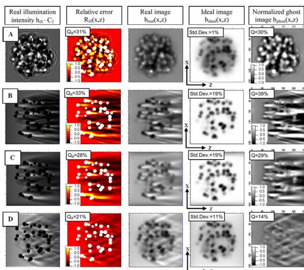
Fig. 3. (Color online) Illumination and imaging with a plane wave (Type A), a cylindrical beam (Type B), a scanned Gaussian beam (Type C), and a scanned Bessel beam (Type D).
