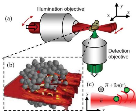
Fig. 1. (Color online) (a) Illumination along  $z$  and detection in  $y$  in a 90° arrangement. (b) Magnification of a light-sheet propagating through a cluster of spheres. (c) Scheme for illumination and scattering at spheres with index  $n(r)$ . Illuminated spheres are green.
