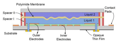
A conceptual depiction of the optofluidic phase modulator to be developed in this project.
