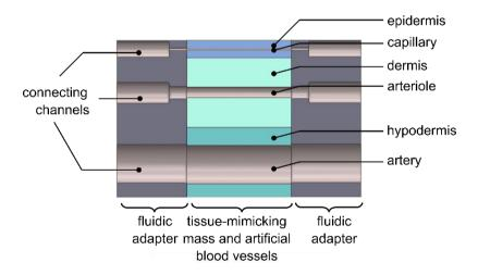
For a new application scenario, we are now looking for a highly motivated Bachelor student that will adapt the existing tissue phantom. Modifications include the change of the phantom geometry by increasing the layer thicknesses, the design of a new fluidic adapter and the characterization of the new tissue phantom.
