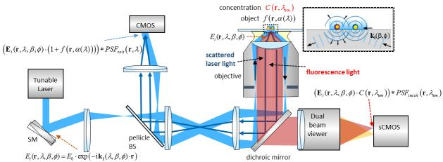
Schematic of a ROCS imaging system: Partially coherent images from back-scattered laser light are combined by rotation in the azimuthal angle  $\phi$  change with the incident k-vector, which can be controlled by the the laser wavelength  $\lambda$  and the polar angle  $\beta$  of incidence. Fluorophores delay the phase of the backscattered laser light and emit fluorescence light at the same time for object identification and control.
