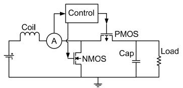
Figure 1: Illustration of a current controlled boost converter
