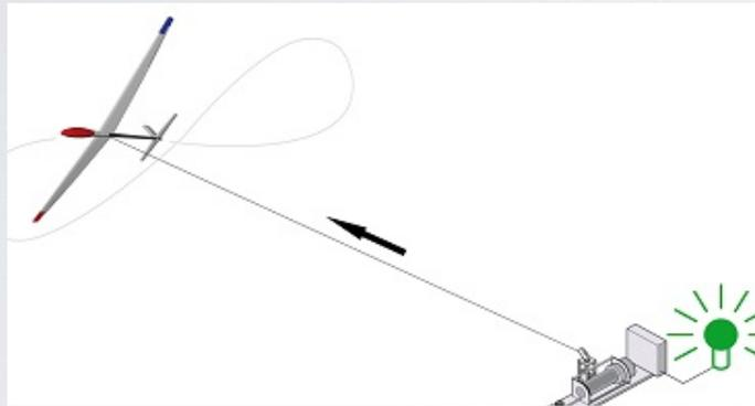
Note: kite flies much faster than wind speed, depending on its aerodynamic efficiency. The faster, the more tension force in the line.
