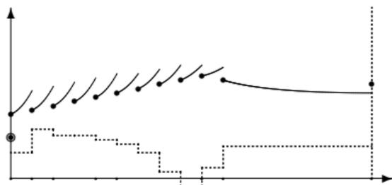
$$\underset{s, q}{\text{minimize}} \quad \sum_{i=0}^{N-1} l_i(s_i, q_i) + E(s_N)$$
