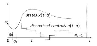
Use numerical integration to obtain state as function x(t; q) of finitely many control parameters  $q = (q_0, q_1, \dots, q_{N-1})$
