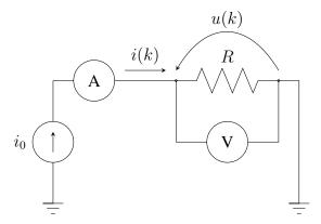
The resistor R has a current  $i_0$  flowing through it which is determined by the current source. The goal of the experiment is to estimate the value of R using Ohm's law. Since the value of  $i_0$  is not known exactly, we use an ammeter to measure the current i(k) and a voltmeter to measure u(k). Since several measurements are taken, k represents the measurement number. We assume that the measurements are noisy:
